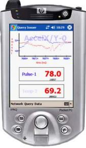
Figure 4: A GUI displays accelerometer data, patient pulse-rate, and environmental temperature.
