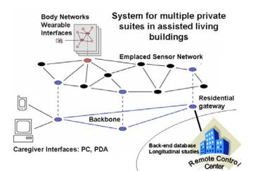
Figure 2: Multi-tiered system architecture, showing physical connectivity.
