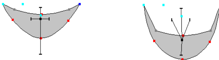
Figure 8. A point skeleton component with two frozen body points (indicated by arrows). Neutral shape (left) and deformed shape (right).
